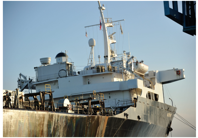
HORIZON SPIRIT showing the radar van (with two radars on top) on the left and the ops van on the right. Photo: courtesy of Ernie R. Lewis, Lead investigator of MAGIC
