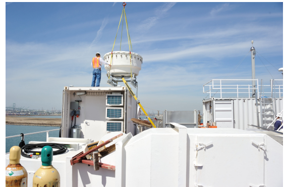
Unknown dock worker aligning radar being loaded on radar van on HORIZON SPIRIT. Photo: courtesy of Ernie R. Lewis, Lead investigator of MAGIC
