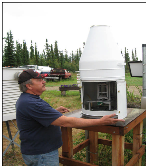
Ron Stuvek servicing a Fischer Porter. One of many Ron maintained during his 36 years at the Fairbanks WFO
