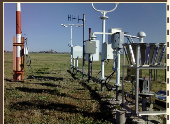
Above: Boston Logan Airport Automated Surface Observing System (ASOS).
