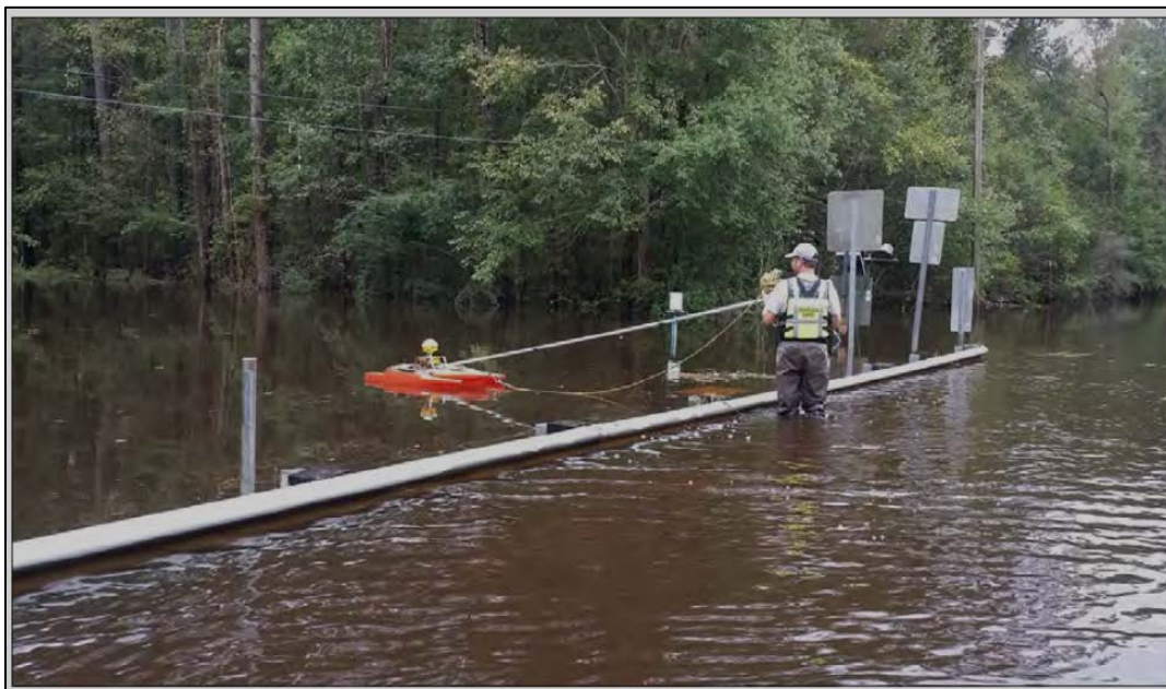
Figure 36: USGS personnel measuring streamflow in Conway, SC. Source: USGS
