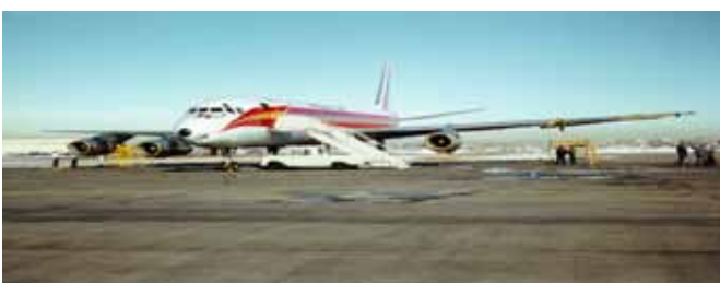
Figures 2-3: American International Airways' DC-8 aircraft after losing its No. 1 engine due to mountain wave turbulence, Dec. 9, 1992. Photos courtesy of Northwest Airlines.
