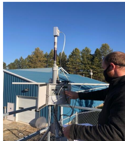
Kelby Sullins from the Idaho Department of Environmental Quality setting up the portable air monitoring station.
